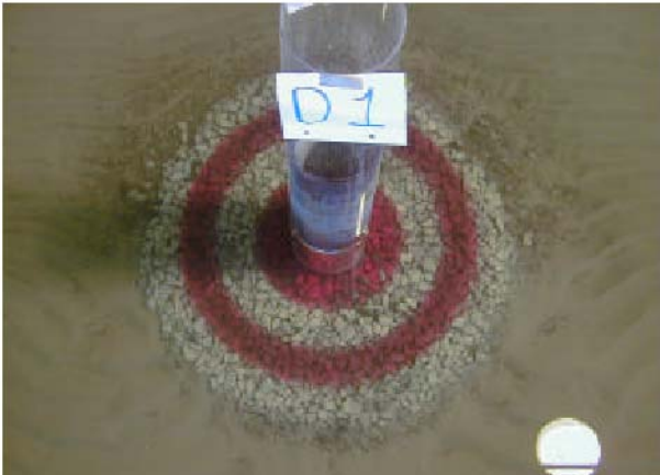
Physical experiment: d_{50} = 0,016\text{m} ( 0,4\text{m} original)
