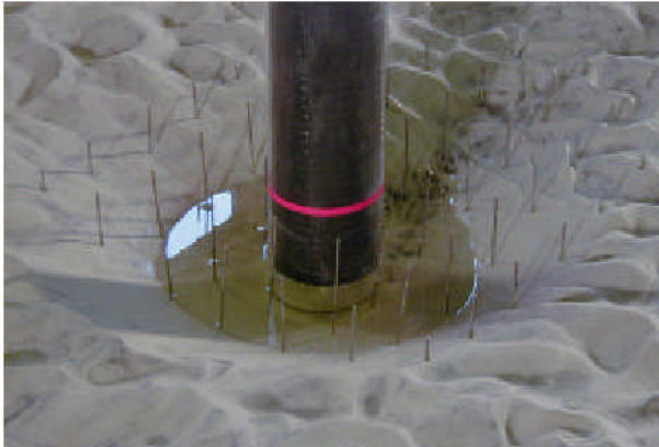
Physical experiment: erosion around an unprotected pile (Horns Rev)
