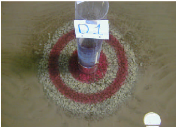
Physical experiment: d_{50} = 0,016\text{m} ( 0,4\text{m} original)
