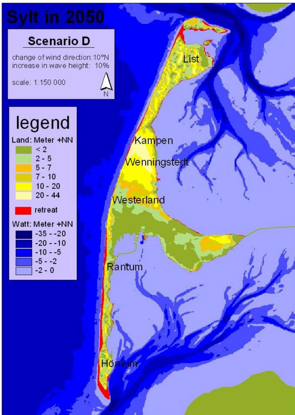
Fig. 7: Coastal retreat in the year 2050, changing the wave direction 10° to north with an increasing wave height of 10%
