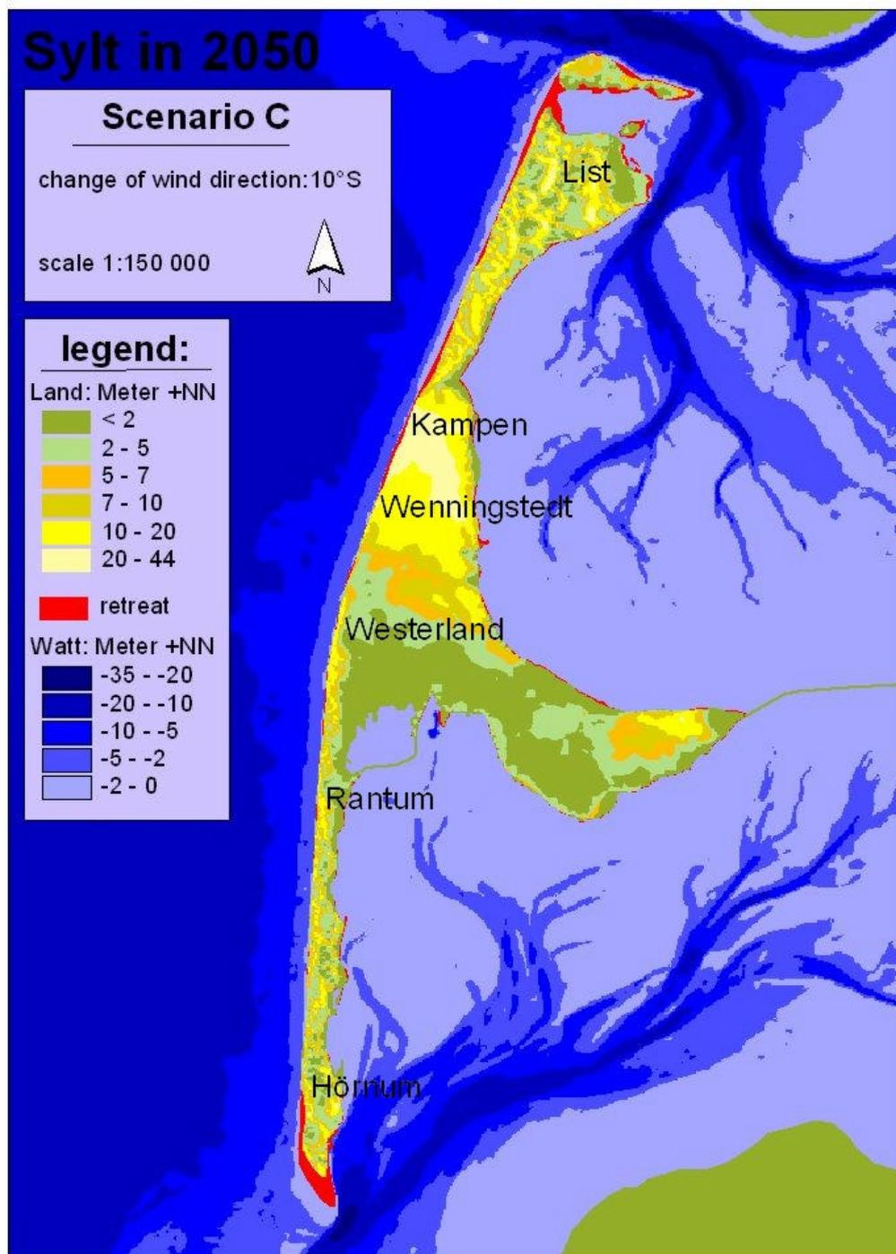
Fig. 6: Coastal retreat in the year 2050, changing the wave direction 10° to south
