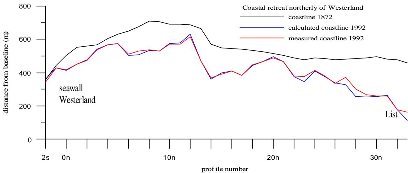
Fig. 5: Calibration of the model for the part northerly of Westerland
