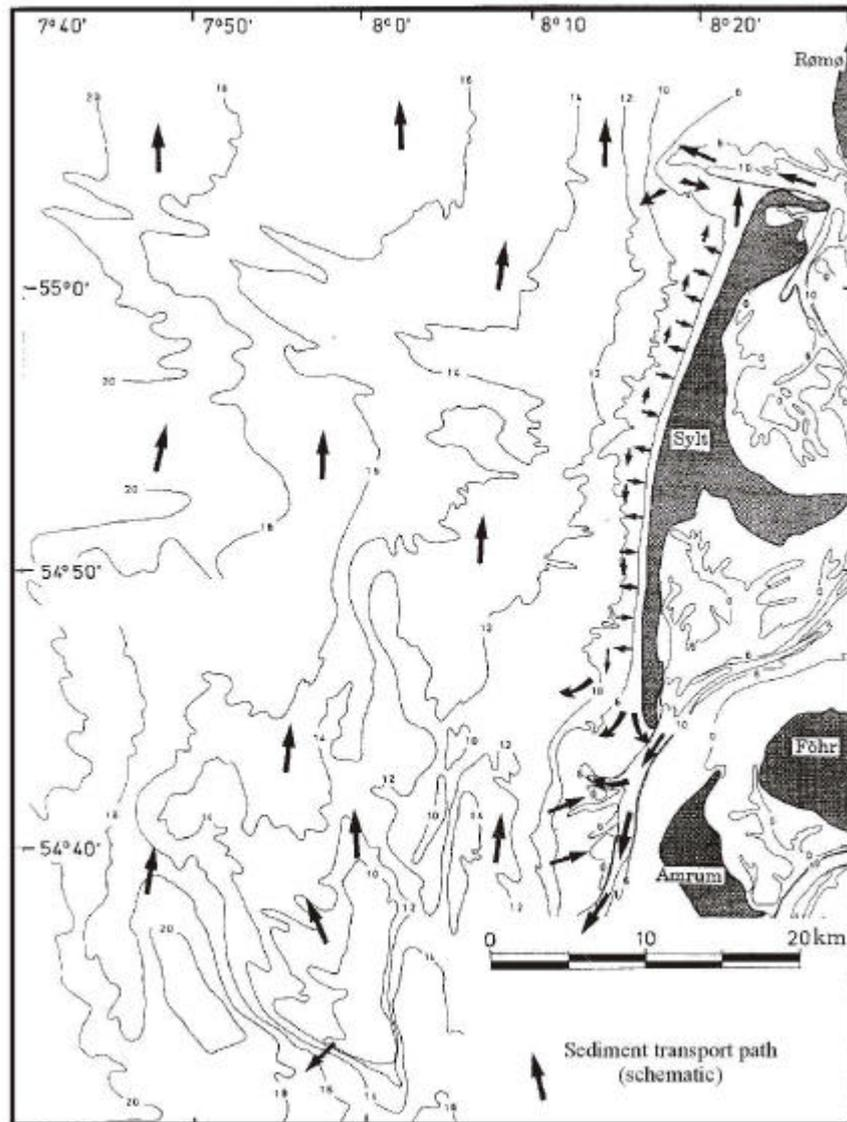
Fig 3: Sediment transport around Sylt (schematic)
